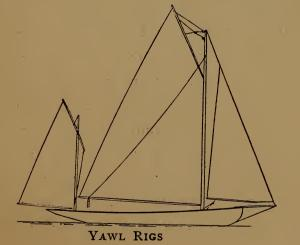
the mast is frequently too short; consequently the head of the sail cannot be kept in place. With jib-headed mizzens the same spar is too light; in consequence when the sheet is brought down hard the mast buckles aft, throwing the head of the sail into a bag. How frequently you see a yawl on the wind with her mizzen all a-shiver. If you make the boomkin longer, the boom stouter, and give the mast a good head, you will get a better sitting and more efficient sail.
